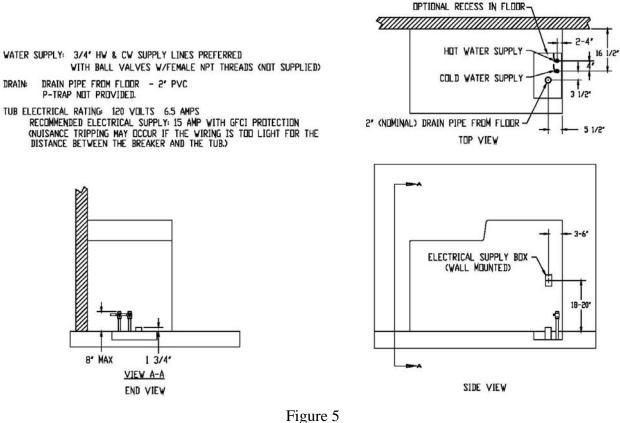
Rough-in Specifications Peninsula Installation – 1 wall – Side plumbing from the floor (Reference figure 1)
