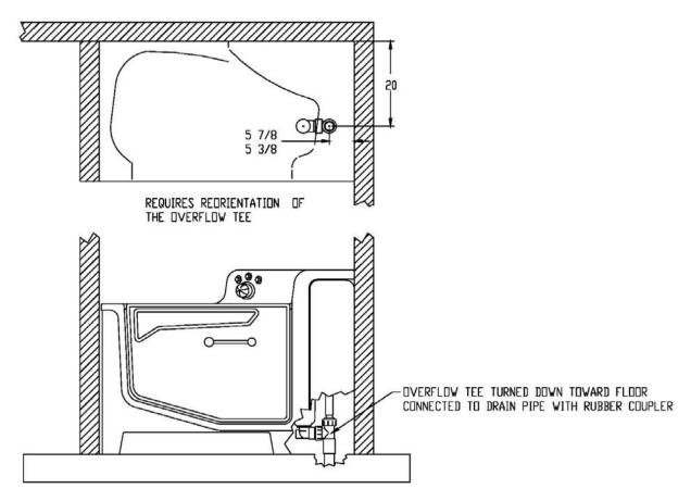
Figure 9 Drain pipe from floor at 20" location.
