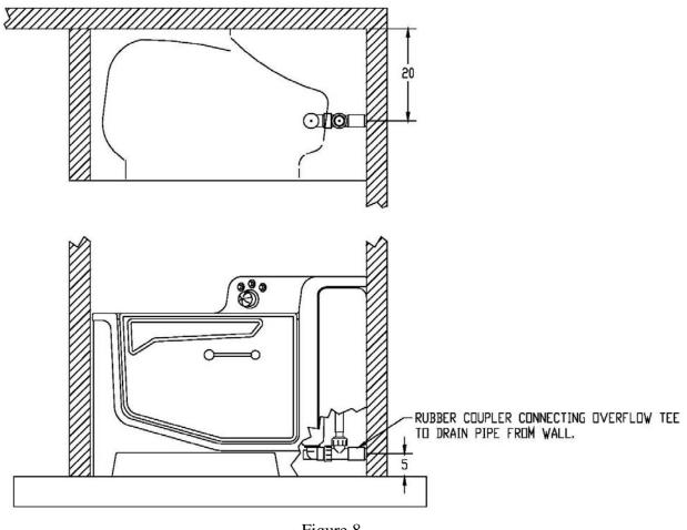
Figure 8 Drain pipe from the wall.
