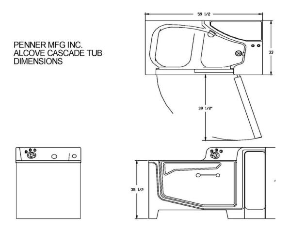
Figure 3 Basic Dimensions Cascade Alcove
