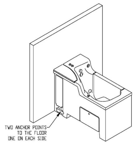
Figure 13 Anchoring Peninsula Installation - 1 Wall - Back
