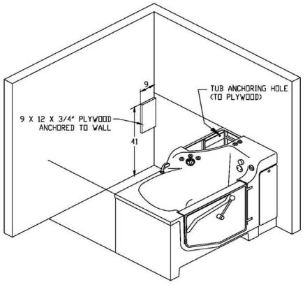
Figure 12 Anchoring Alcove Installation - 2 or 3 Walls
