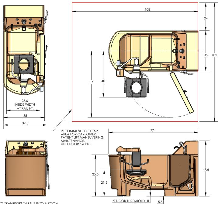
TO TRANSPORT THIS TUB INTO A ROOM, THE DOOR OPENING WIDTH MUST BE 38 INCHES. HOWEVER, IT CAN BE AS SMALL AS 35 INCHES IF THE WATER DOOR AND SHOWER ELBOW ARE REMOVED FROM THE TUB PRIOR TO ENTRY.
