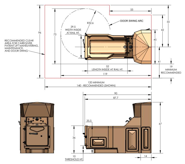
35 1/2 INCH DOOR OPENING REQUIRED FOR TUB ENTRY INTO ROOM
