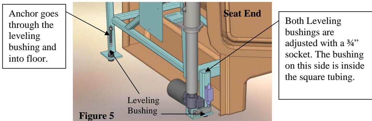
2. Remove the end panel, at the seat end of the tub, and set it to the side.
